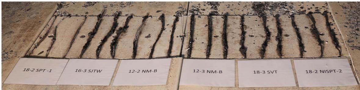
Figure 5.1: Photograph of the 18 cord exposures in the test room following Experiment 2. The placards identify the cord type.
