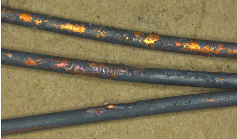
Figure 5.2: Magnified photograph of the 12-2 NM-B cable on a thermal magnetic circuit breaker following Experiment 2 showing both a bead and a notch on the cable.
