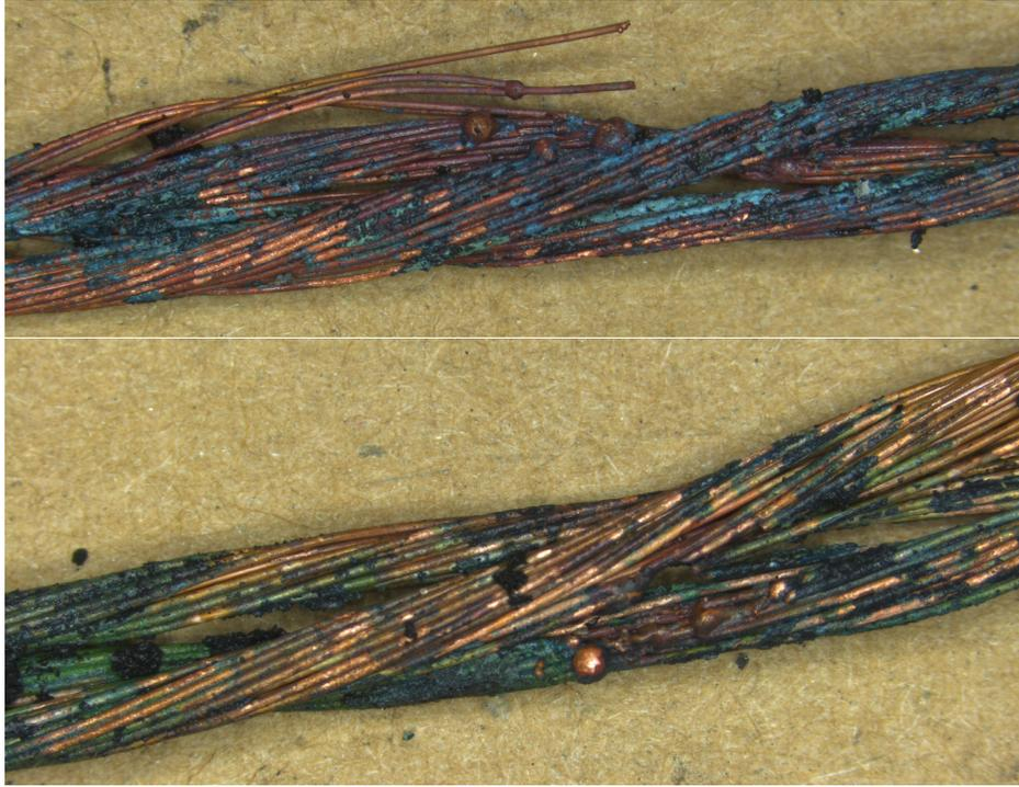
Figure 5.3: Magnified photograph of the 16-3 SJTW cord on a thermal magnetic circuit breaker following Experiment 1 (top) and Experiment 5 (bottom).
