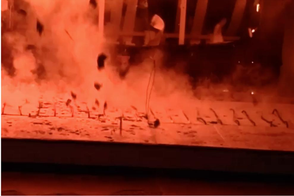
Figure 4.5: Experiment 1 – Debris falling from ceiling onto heat flux gauge 3.
