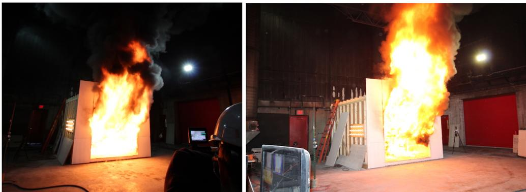
Figure 4.2: Photographs of the room during flashover, prior to any of the circuits tripping - Experiment 5 (left) and Experiment 6 (right).
